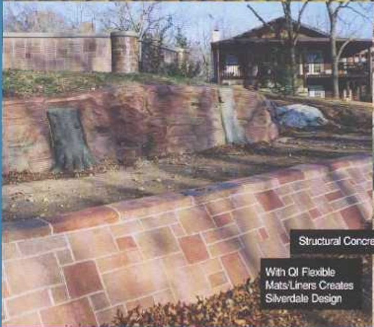
QI Designed Rock Cleft & Trees, Sculpted in Place - No Forms. 500PSI Concrete, 1750 lbs Sand, 1320 3/4 Aggregate, 496 lbs Cement, 74 lbs Fly Ash, No Water Reducer
